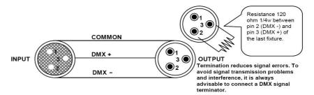
**Caution:** Do not allow contact between the common and the ficture's chassis ground. Grounding the common can cause a ground loop, and your fixture may perform erratically. Test cables with an ohm meter to verify correct polarity and to make sure the pins are not grounded or shorted to the shild or each other.
