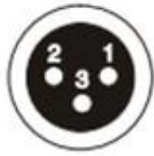
DMX output XLR Mounting socket
