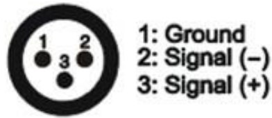
DMX Input XLR Mounting plug
